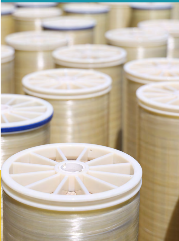
Arlington Desalter reverse osmosis membranes
