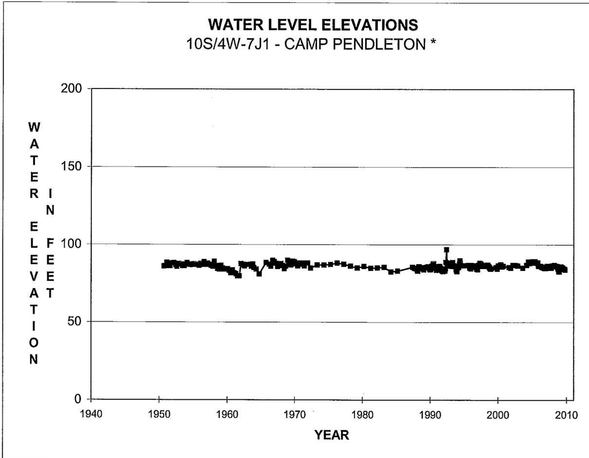
Ground El. 92 Feet; Depth 141 Feet; Perf. Unknown; Drilled in Alluvium
