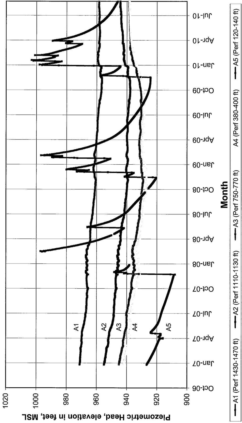
**End-of Month Piezometric Head for Multiple Depth Monitoring Well
