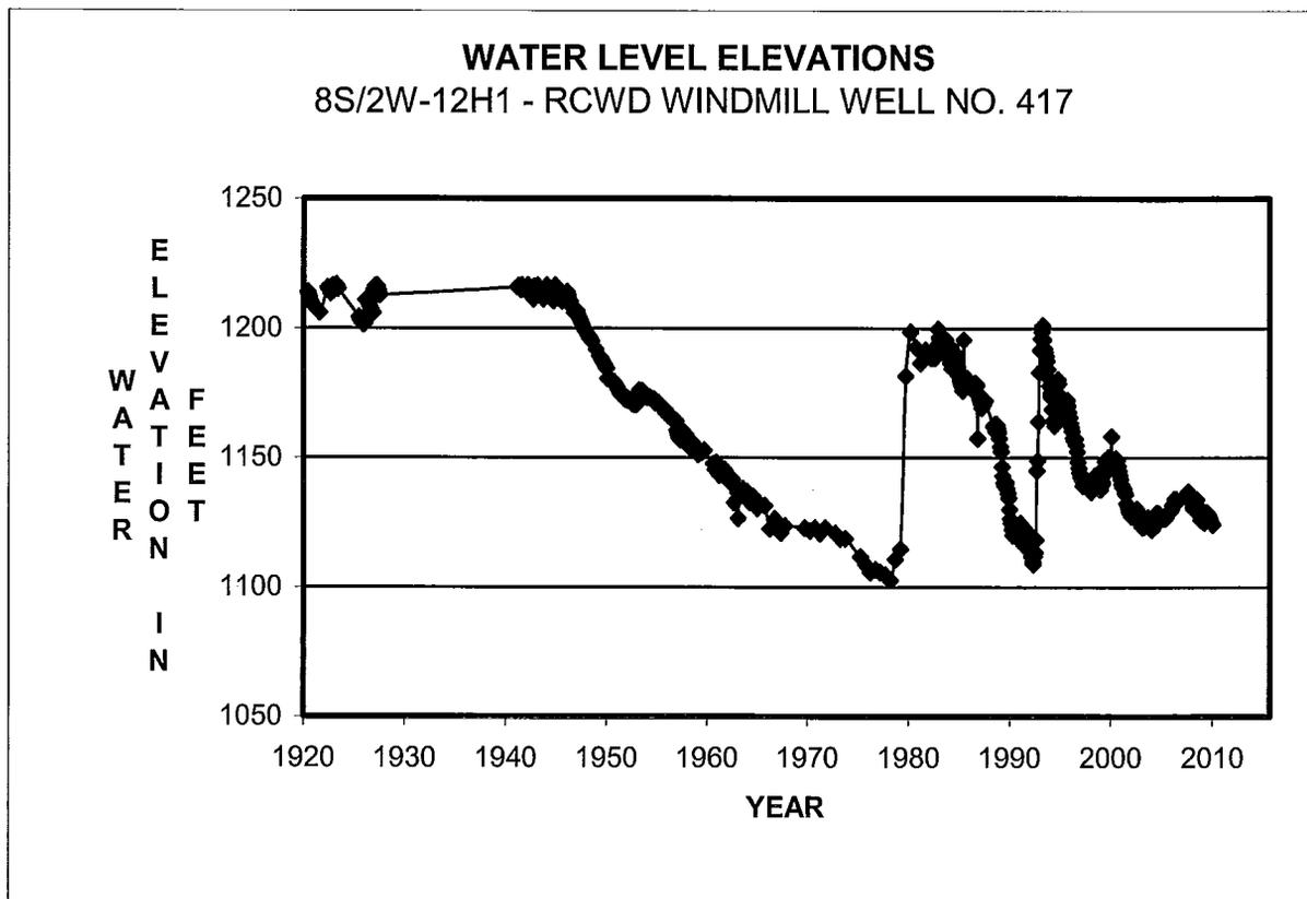
Collar El. 1216.7 Feet; Depth 515 Feet; Drilled in Alluvium
